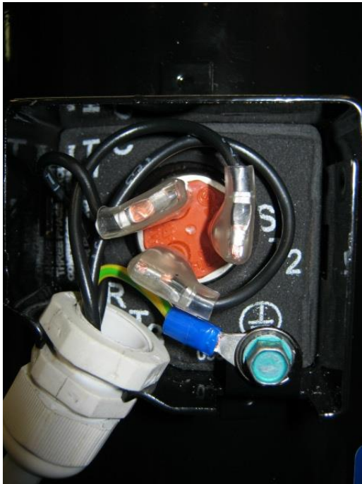
Figure 14: Correct electrical installation with cable glands for IP21 T-box (models ZB15K* to ZB45K*)
