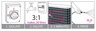
To use SuperClean™ as a heavy duty, foaming cleaner for aluminium-finned, air-cooled condensers, dilute with 3 parts water. Using a low pressure sprayer, spray between the fins – starting at the bottom in one corner and progressing methodically across and up. Cleaning is more effective if coil is still warm. In minutes a heavy foam will form, forcing contamination outwards. Foam and contamination must then be rinsed away thoroughly with fresh water.
